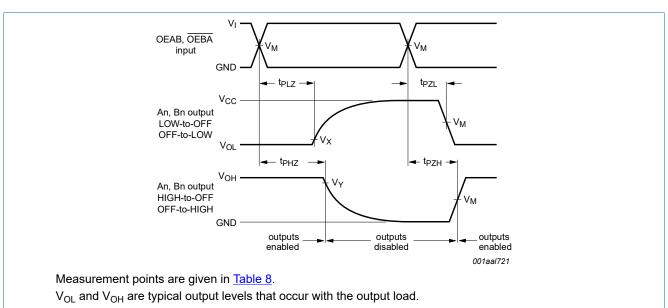
Fig. 6. 3-state output enable and disable times
